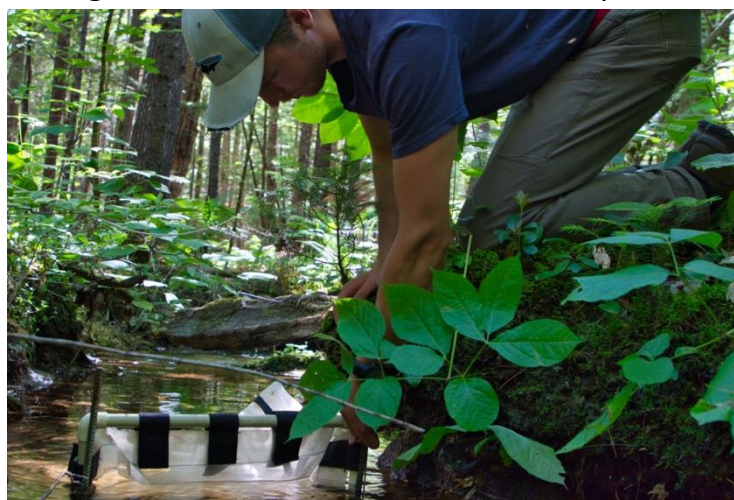
Tin Mountain intern Donovan Spaulding sets up a surber sampler in Black Brook that will be left overnight
